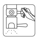
Turn on the filling tap and release the pressure
